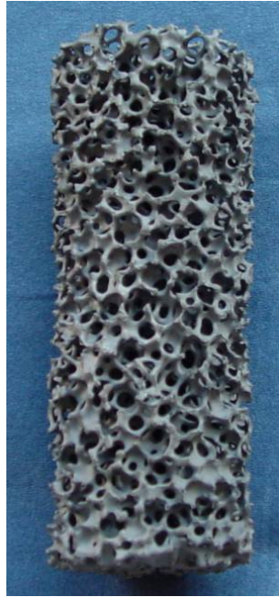
Poröse Brennzone (SiC-Schaum)
